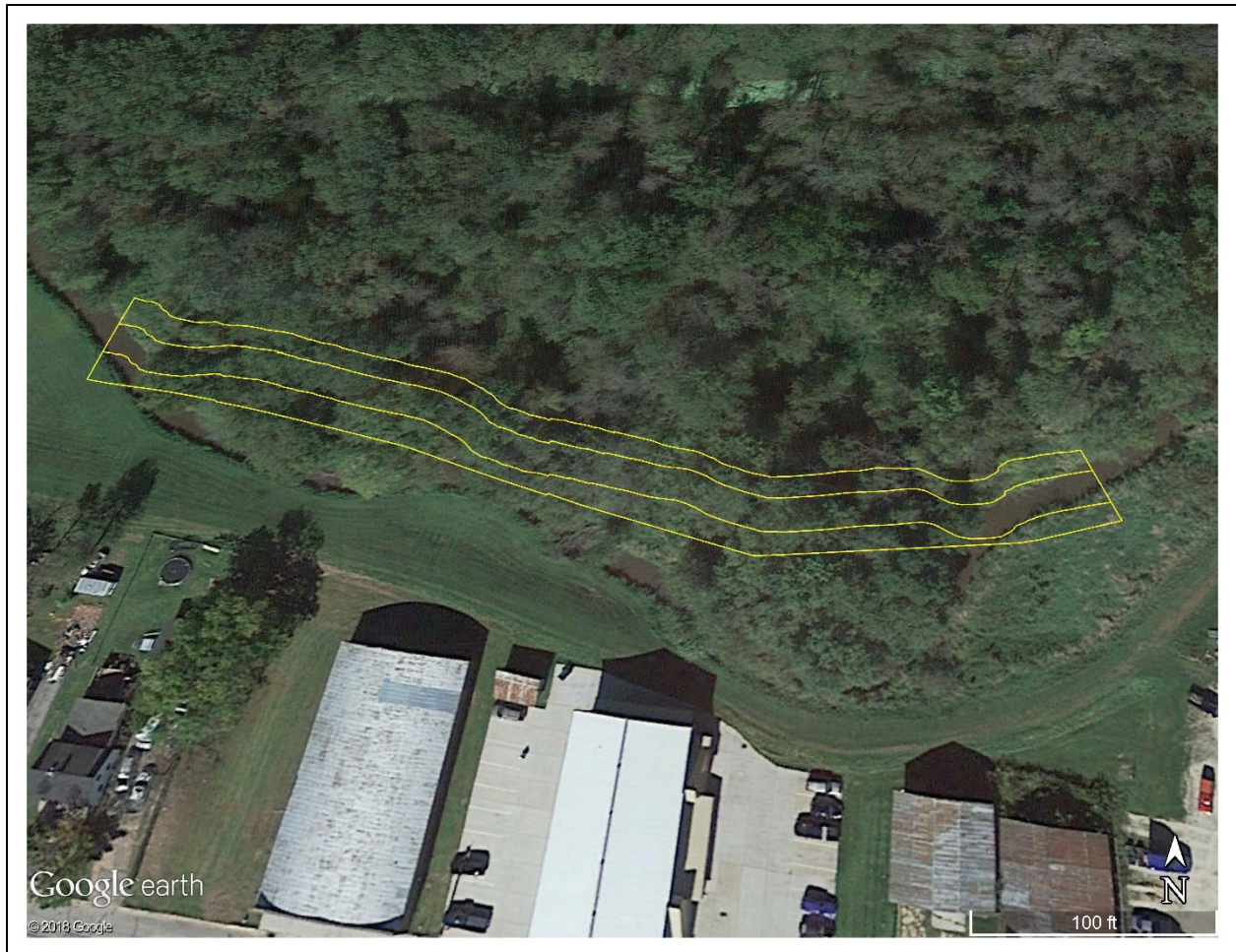
Figure 2. Turton Creek reroute in Reach 2. Existing channel is 642 linear feet and the new channel (yellow) would be 564 linear feet (loss of 78 linear feet).
