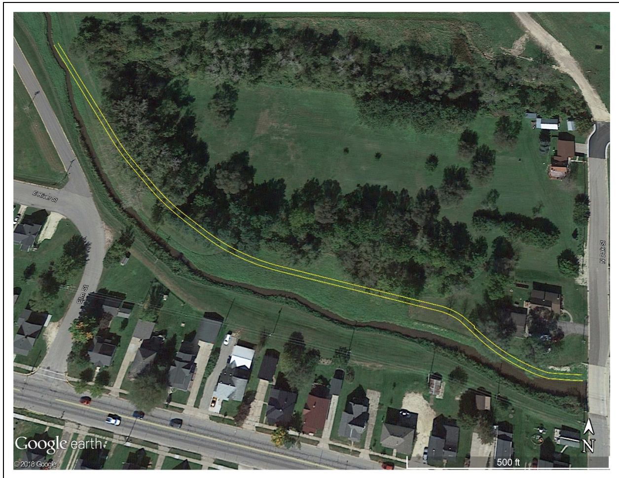
Figure 1. Turton Creek reroute in Reach 1. Existing channel is 1,100 linear feet and the new channel (yellow) would be 1,067 linear feet (loss of 33 linear feet).
